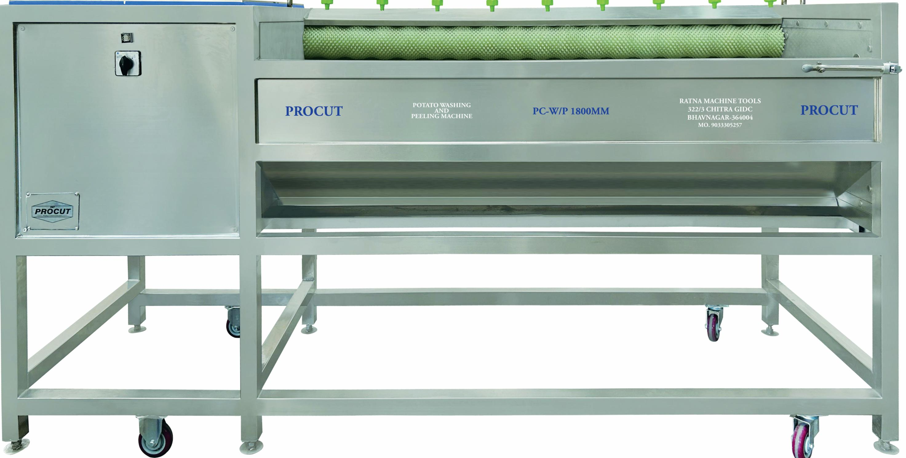
**PC-W/P** is designed to change the conventional method of peeling the **potatoes**, **onions, Ginger & Carrot etc.** It comes with **Nylon Fiber F6** Material of **brush rolls** which peels the components from all angle with **peeling accuracy** of **95%**. It has biult in Spray Jet to wash the vegetables while peeling process.
